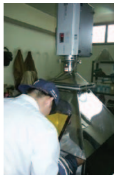
30 sec arc on time with 5 minute continuous fume collection
