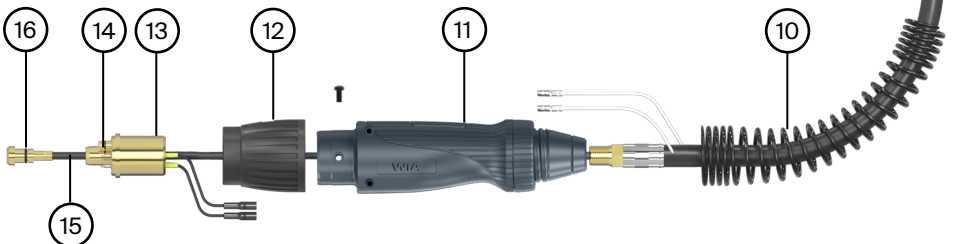
Fig 8 300 Amp Torch Supplied with Weldmatic 350. Use Centre Fire Tip Consumables.
