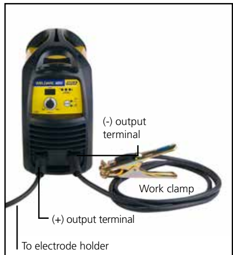
Fig 3 Connections for Stick Welding (MMAW), Electrode Positive
